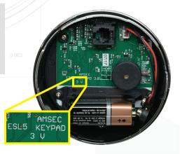
**KEYPAD** - "3 V" is visible on the circuit board (see photo above)
