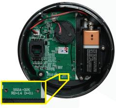
**KEYPAD** - "R2=1.4" is visible on the circuit board (see photo above)
