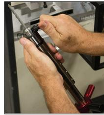
4c. Closing chuck with Drill Bit in position.
