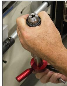
4a. Holding the chuck collar and rotating the chuck sleeve counterclockwise.
