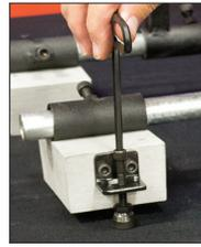
3d. Extending the jack screw on the Magnetic Foot.
