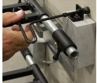
3j. Retracting the jack screws on the Magnetic Feet Tubes to insure the frame is secure on the Safe or Vault door.
