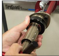
6d. Slide the Barrel and Quill Assembly into the Quick Release Coupling; align the red dot on the coupling with the indents on the Barrel.
