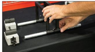
3b. Placing the pipes (2) through the Frame Tubes.
