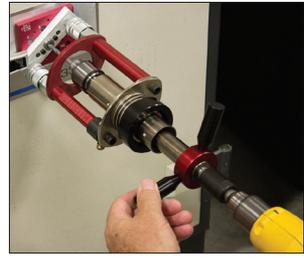
8a. Start the drill motor and feed the bit into the safe using the end cap handles.
