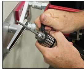
6c. Using the chuck key, tighten in all three positions.
