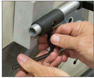
3i. Loosening the cap screws on the Magnetic Feet Tubes.
