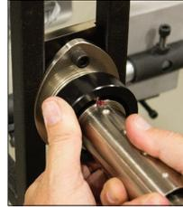
4d. Sliding and aligning the Barrel & Quill Assembly.
