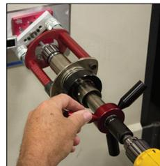
7b. Insert the nut driver into the hex drive socket, now you are ready to penetrate the safe.
