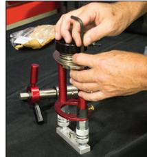
3f. Removing the Coupling from the Barrel Assembly.
