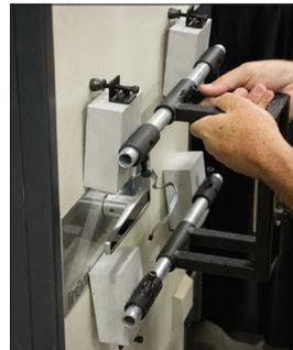
3h. Placing the assembled Drill Rig Frame on the Safe or Vault Door.
