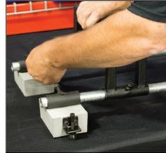
3e. Tightening the cap screws on each foot.
