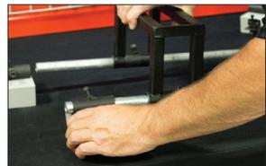
3c. Placing the Magnetic Feet (4) on the Pipes.
